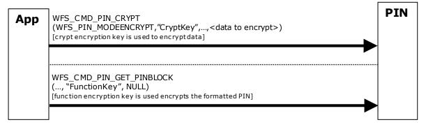
Master key restriction disallows loading of derived keys with different usage:
